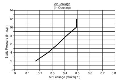
Air leakage chart is based upon independent air leakage tests conducted by Architectural Testing Laboratory. The out-opening model of a 24" x 60" AHF-T4 was tested. Tests were in accordance with ASTM E 283-91 "Determining the Rate of Air Leakage through Exterior Windows, Curtain Walls, and Door under Specified Pressure Differences Across the Specimen". Air Balance recommends using out of opening doors for draw through applications and in opening (IO) for blow through applications.
